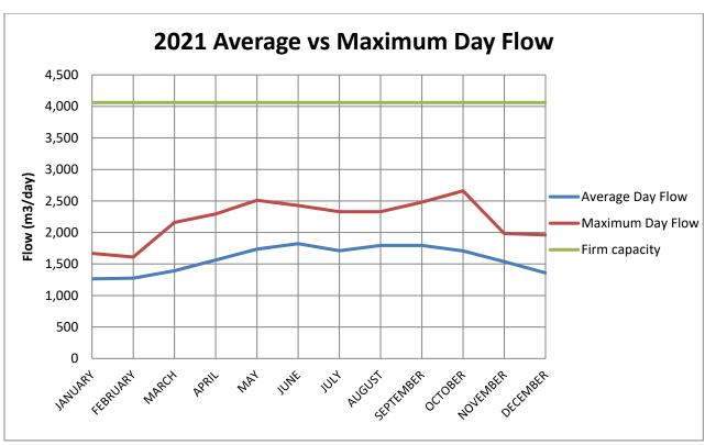
Tavistock Firm Capacity 4,061 m<sup>3</sup>/day Tavistock Water Supply Capacity 5,616 m<sup>3</sup>/day
