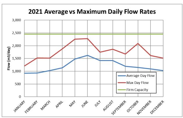
Oxford South Water System Firm Capacity 2,454 m³/day Oxford South Water System Capacity 6,054 m3 /day
